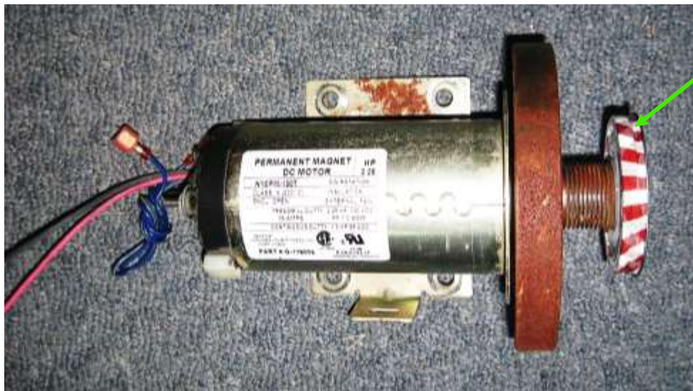
Figure 11: the jar lid to prevent the belt from sliding off the generator shaft
