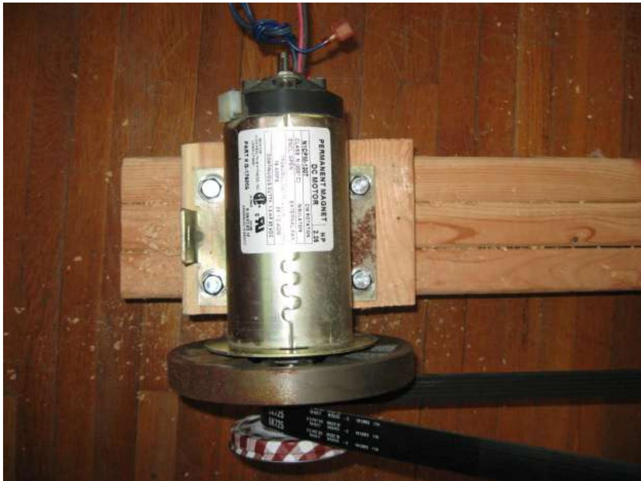
Figure 10: the generator bolted to its platform
